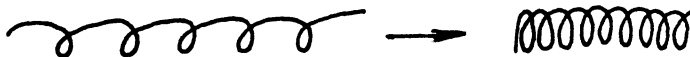
Fig.5. The extended helix is contracted to a tight-helix upon inclusion complex formation - e.g. with iodine.
